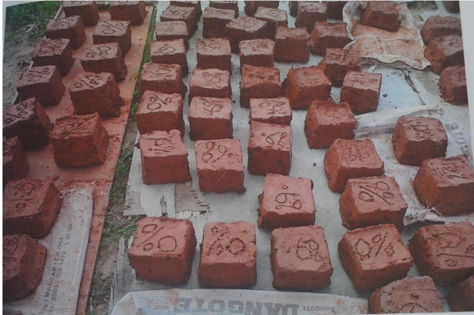
Plate 1. Coir reinforced laterite blocks under curing.
