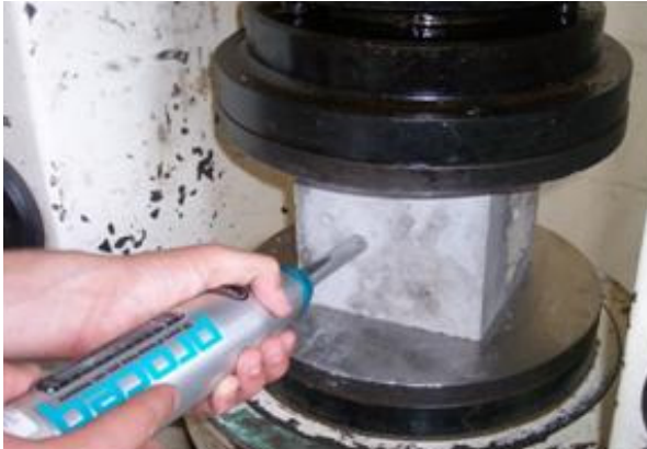
Figure 1. The cube specimen placed in the testing machine.
