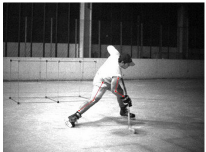
Figure 3. Marker positions and segments created.
