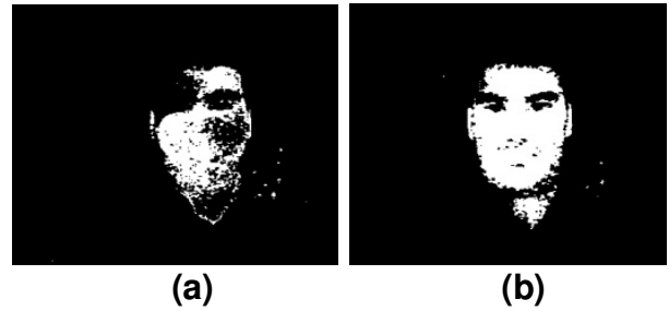
Figure 8. Comparison of skin color identification algorithms: (a) RGB coding technique; (b) YCbCr coding technique.
