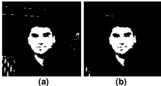
Figure 6. Application of the median filter: (a) Image with photo noise; (b) Image free of noise.
