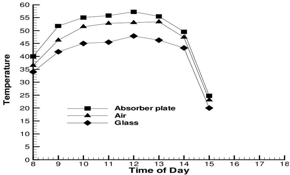
Figure 3b. Temperature distribution of the system on a typical day in winter.
