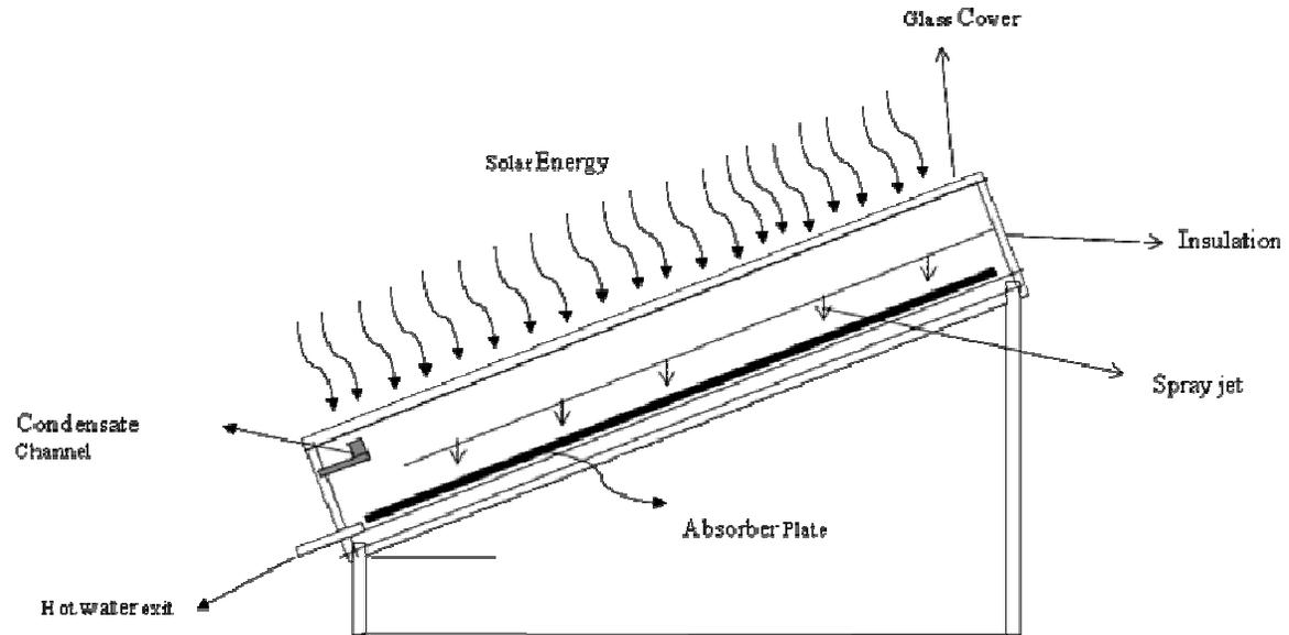
**Figure 1a.** Schematic diagram of the incline solar water distillation system.
