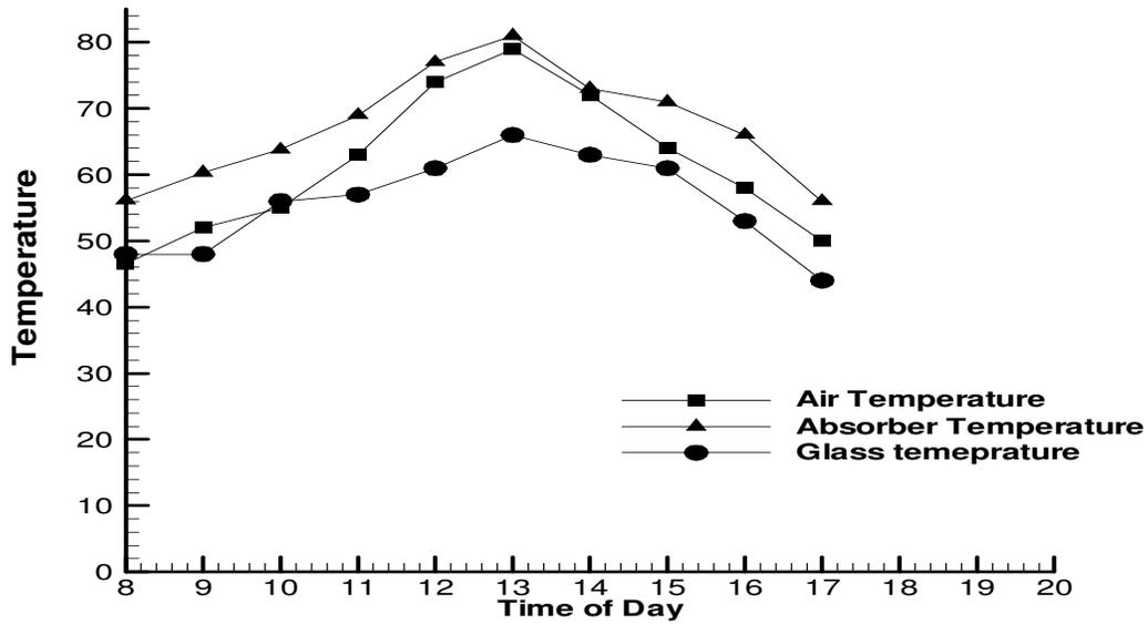
Figure 3a. Temperature distribution of the system on a typical day in summer.
