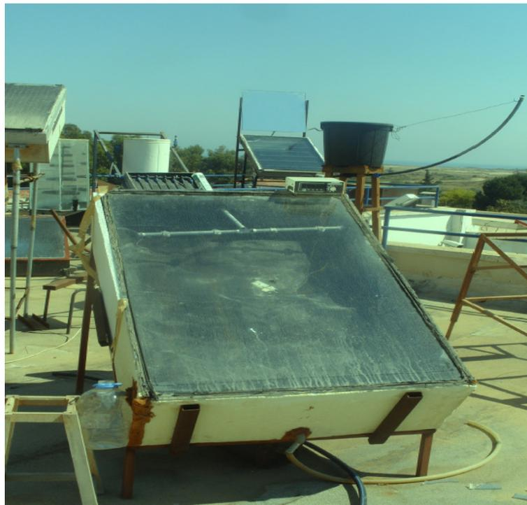
**Figure 1b.** A photograph of the incline solar water distillation system.
