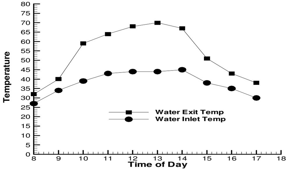
Figure 5a. Inlet and outlet temperature of water on a typical day in summer.
