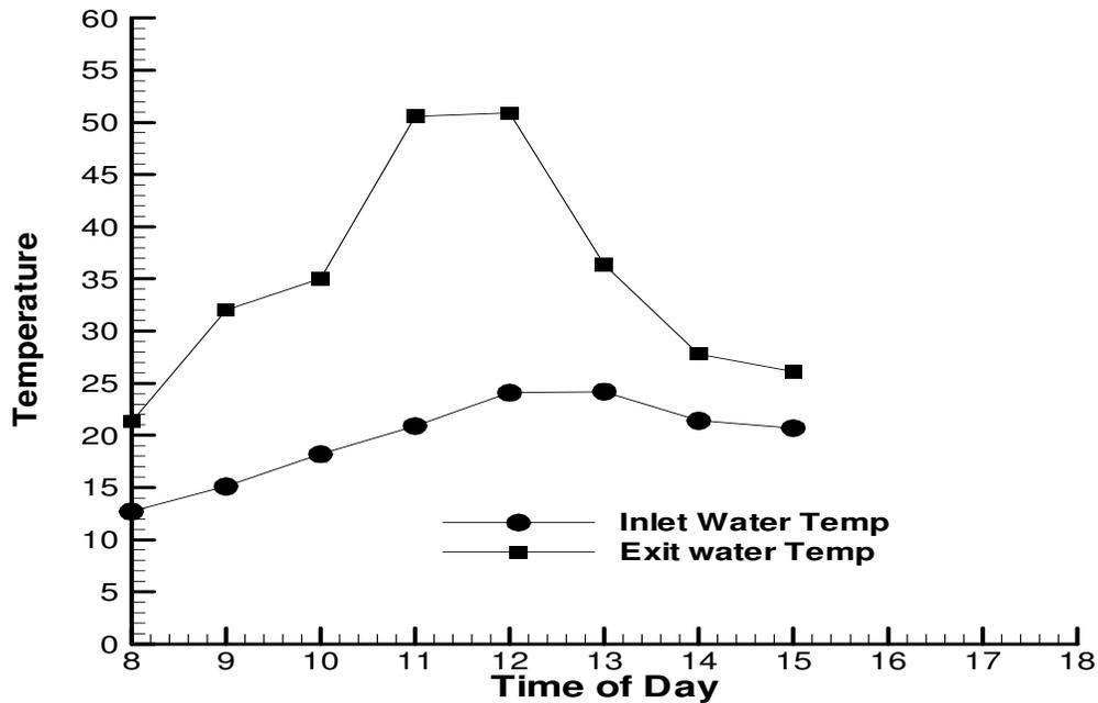
Figure 5b. Inlet and outlet temperature of water on a typical day in winter.
