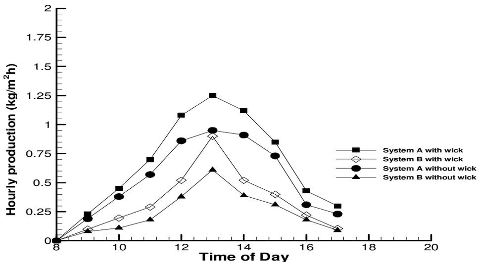
**Figure 7.** Hourly variations of hourly productivity system A (improved ISWD) and system B (older version of ISWD) during summer when both were exposed to the same experimental conditions.
