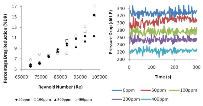
Figure 4. Effect of particle concentration in transported water on Dr% with different Re in 0.0381 n D.I and 2.0 m pipe length and pressure drop analysis for Re = 105000.
