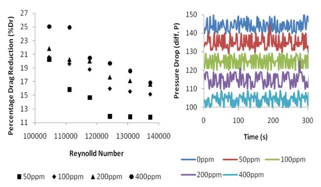
Figure 3. Effect of particle concentration in transported fuel on Dr% with different Re in 0.0381 n D.I and 2.0 m pipe length and pressure drop analysis for Re = 105000.
