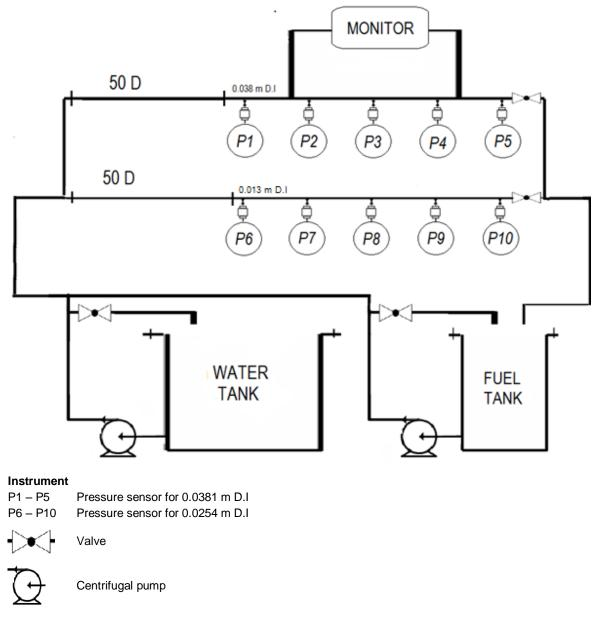
Figure 1. Schematic diagram of the flow system.
