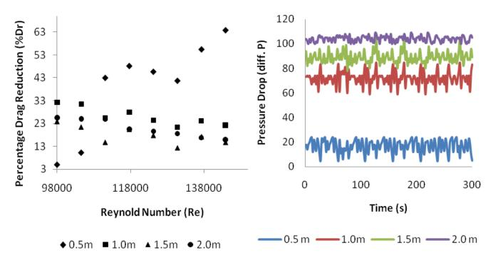
Figure 7. Effect of pipe length in 400 ppm addition concentration flowing in fuel with pipe diameter 0.0381 m D.I and pressure drop data for Re = 139000.
