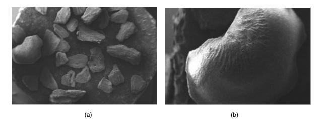
**Figure 2.** Grinded slag waste particle for 200 µm: (a) SEM picture of 9x mag and (b) Scaled up picture of a particle (33x mag).
