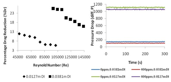
**Figure 5.** Effect of pipe diameter flowing through 2 m pipe length in fuel and 400 ppm concentration addition and pressure drop data for pipe diameter of 0.0127 and 0.0381 m D.I.
