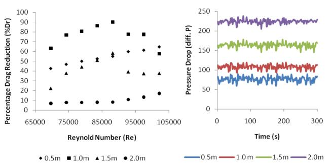
Figure 8. Effect of pipe length in 400 ppm addition concentration flowing in water with pipe diameter 0.0381 m D.I and pressure drop data for Re = 100000.
