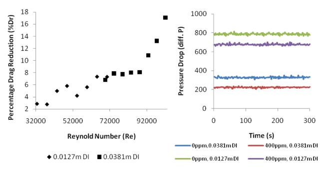
Figure 6. Effect of pipe diameter flowing through 2 m pipe length in water and 400 ppm concentration addition and pressure drop data for pipe diameter of 0.0127 and 0.0381 m D.I.
