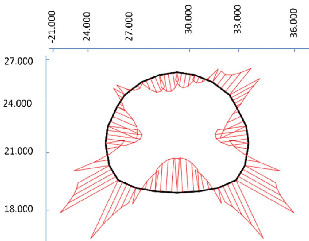
(4E) Vertical displacements (Extreme vertical displacement  $52.32 \times 10^{-3}$  m).
