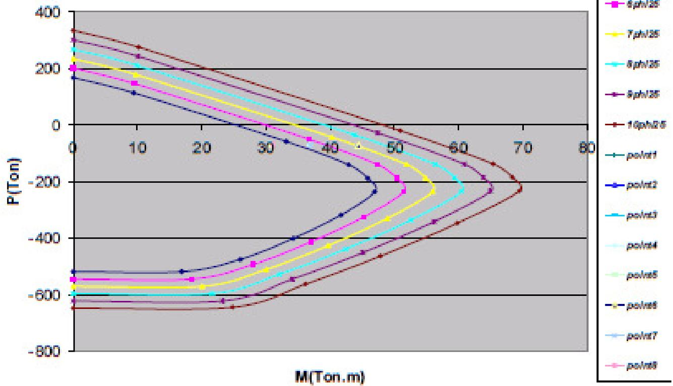
(B) Interaction diagram [M (ton-m) and P (ton)].
