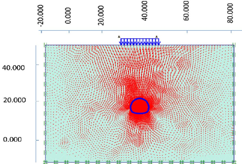
**Figure 5.** PLAXIS outputs for tunnel with 30 m overburden, (A) Typical mesh, (B) Horizontal displacements, (C) Bending moment, (D) Total displacements, and (E) Vertical displacements.
