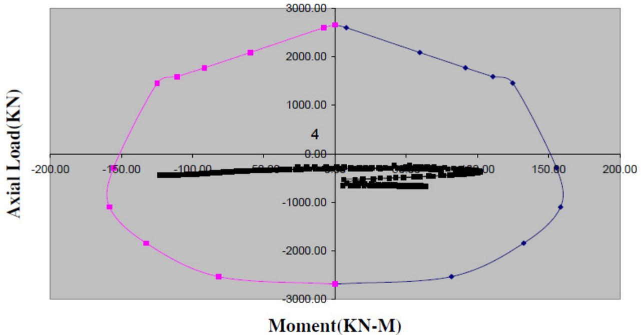
Figure 3. Interaction steel frame (shotcrete = 30 cm, IPE = 200).
