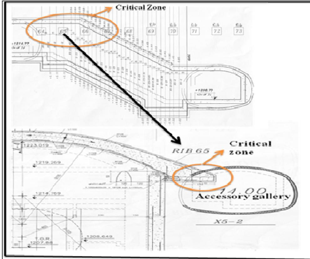
Figure 1. Cross section of metro tunnel showing critical zone of station and access galleries.
