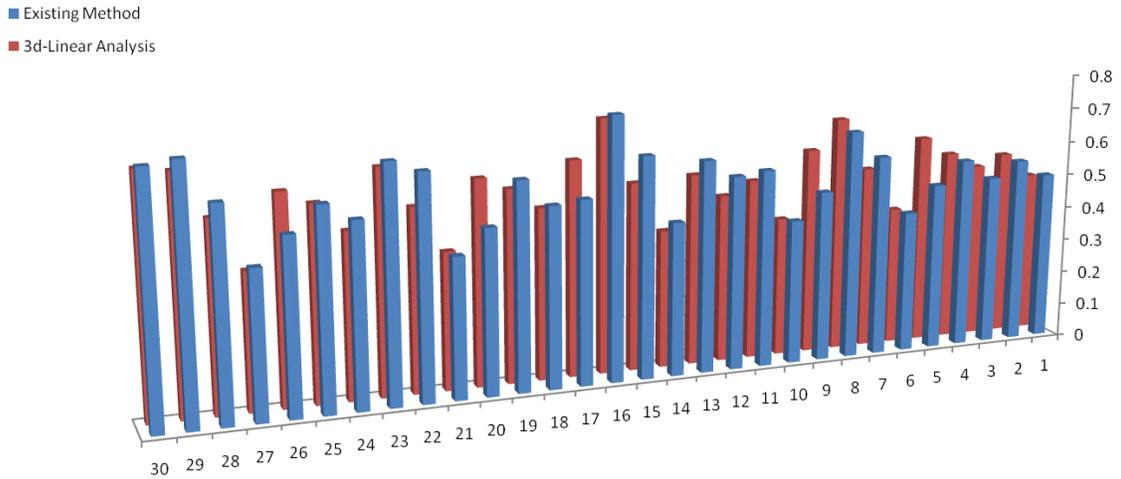
Figure 2. Stress ratio in linear method for pipe bridge (existing method and 3D-linear analysis).
