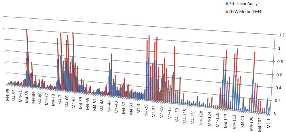
Figure 9. Stress ratio in linear method for piperack M4 (new method and 3D-linear analysis).
