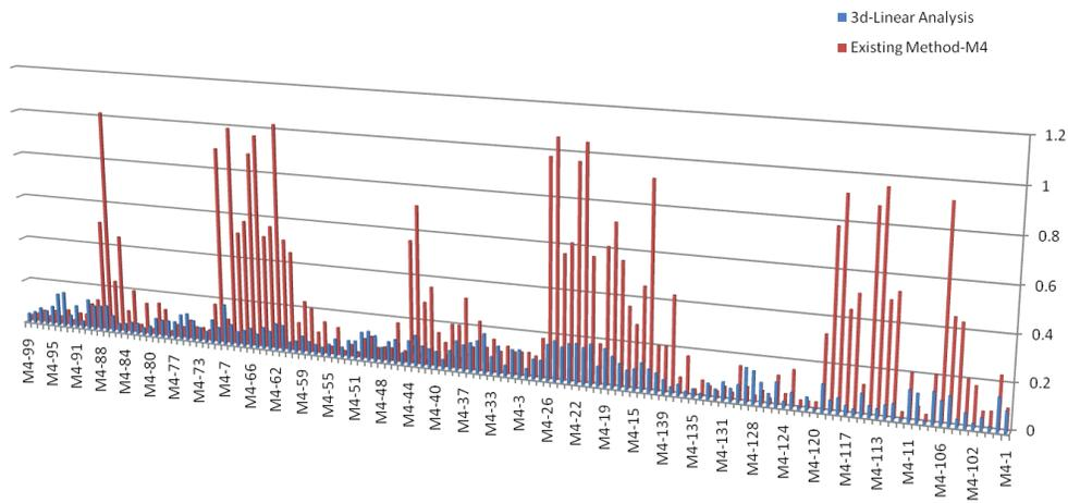
Figure 6. Stress ratio in linear method for piperack M4 (existing method and 3D-linear analysis)
