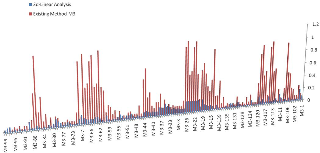
Figure 5. Stress ratio in linear method for piperack M3 (existing method and 3D-linear analysis).
