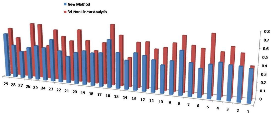
Figure 10. Stress ratio in linear method for pipe bridge (new method and 3D-nonlinear analysis)
