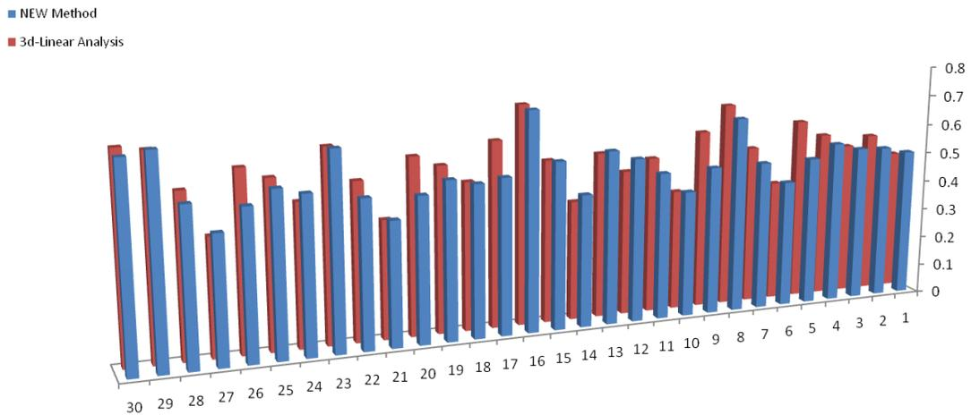
Figure 3. Stress ratio in linear method for pipe bridge (new method and 3D-linear analysis).
