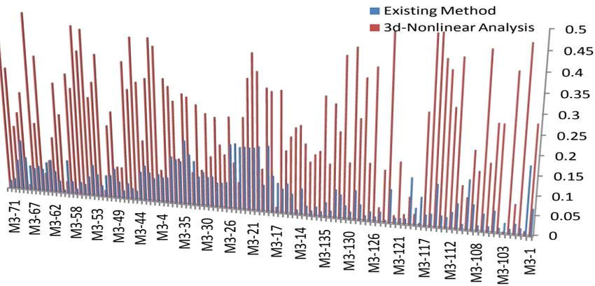
**Figure 12.** Stress ratio in linear method for pipe rack M3 (existing method and 3D-nonlinear analysis).
