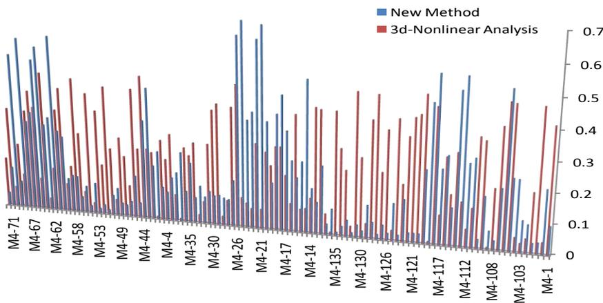
**Figure 16.** Stress ratio in linear method for pipe rack M4 (new method and 3D-nonlinear analysis)
