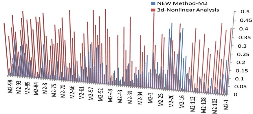
**Figure 14.** Stress ratio in linear method for pipe rack M2 (new method and 3D-nonlinear analysis).
