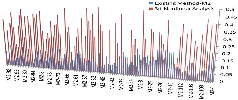
**Figure 11.** Stress ratio in linear method for pipe rack M2 (existing method and 3D-nonlinear analysis)
