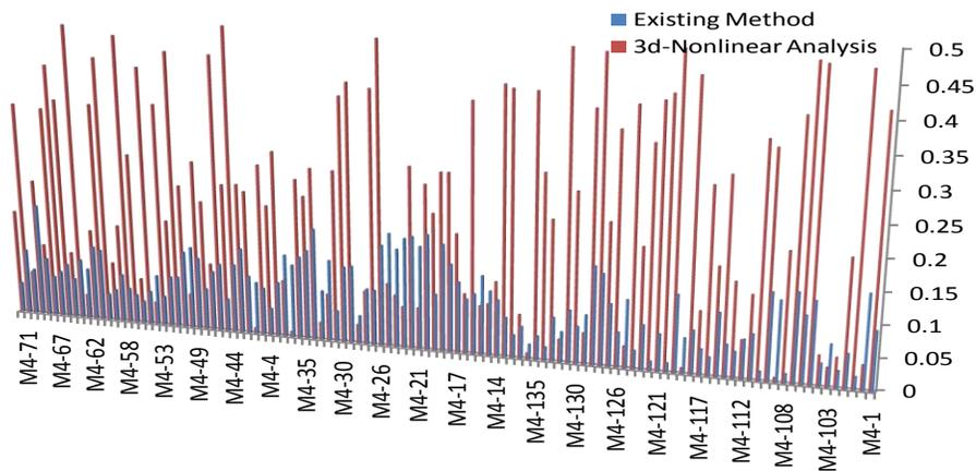
**Figure 13.** Stress ratio in linear method for pipe rack M4 (existing method and 3D-nonlinear analysis).
