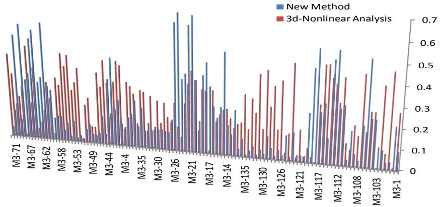
**Figure 15.** Stress ratio in linear method for pipe rack M3 (new method and 3D-nonlinear analysis)
