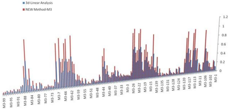
Figure 8. Stress ratio in linear method for piperack M3 (new method and 3D-linear analysis)
