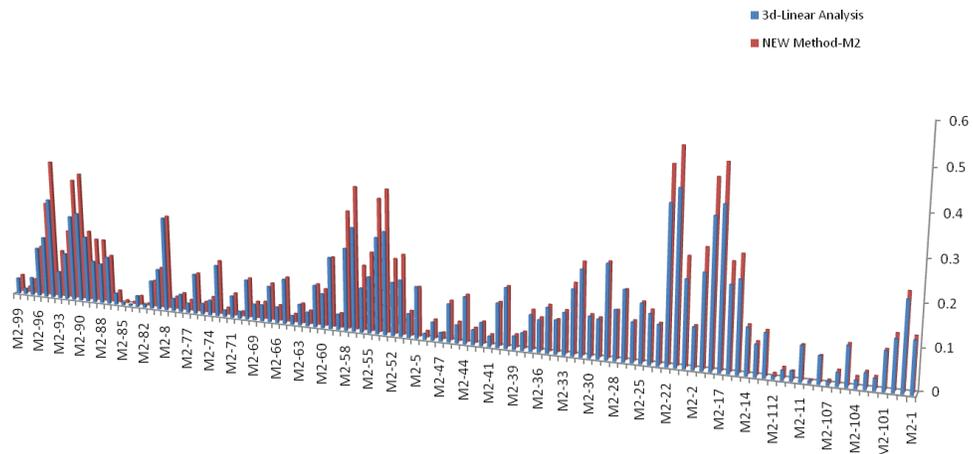
Figure 7. Stress ratio in linear method for piperack M2 (new method and 3D-linear analysis)
