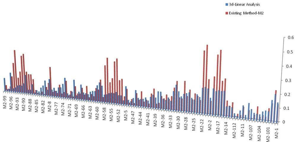
Figure 4. Stress ratio in linear method for piperack M2 (existing method and 3D-linear analysis).
