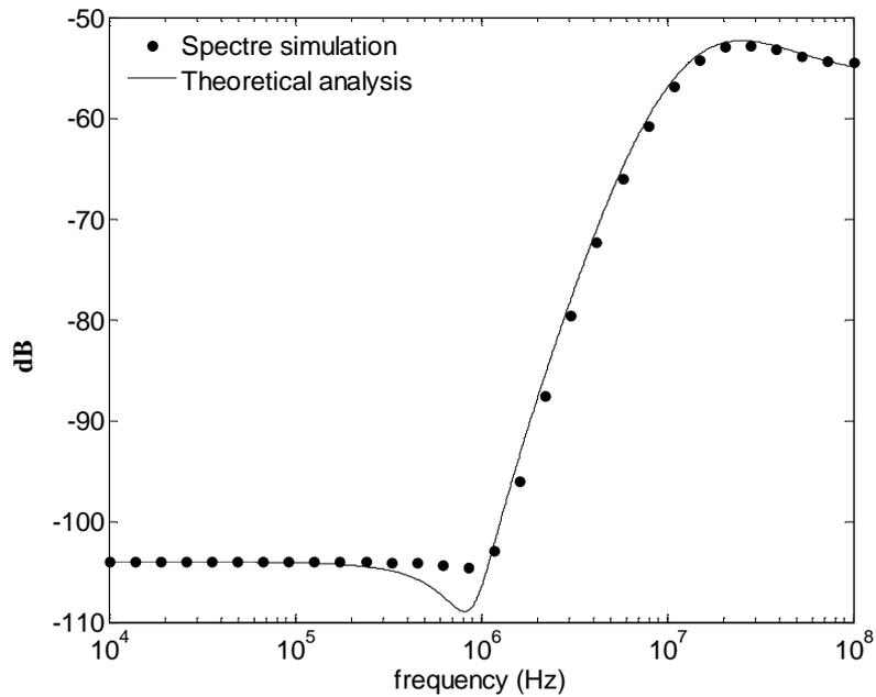
Figure 7. Third-order distortion factor of the cascode amplifier.
