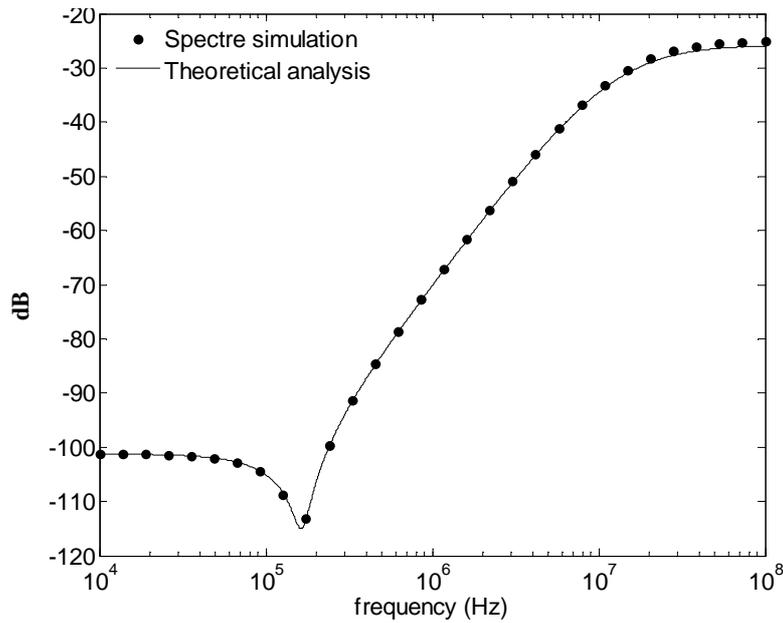
Figure 6. Second-order distortion factor of the cascode amplifier.
