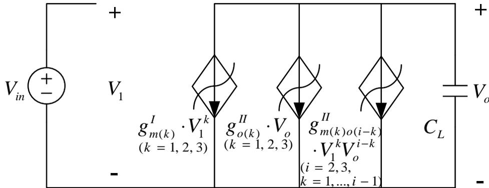
Figure 1. Nonlinear small signal circuit of single stage amplifier.
