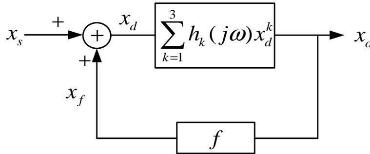
Figure 2. Block diagram of the closed-loop amplifier.
