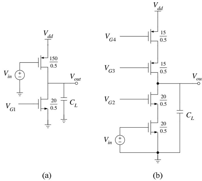
**Figure 3.** (a) Current-sink inverter; (b) cascade amplifier. The unit of transistor dimensions is  $\mu\text{m}$ .
