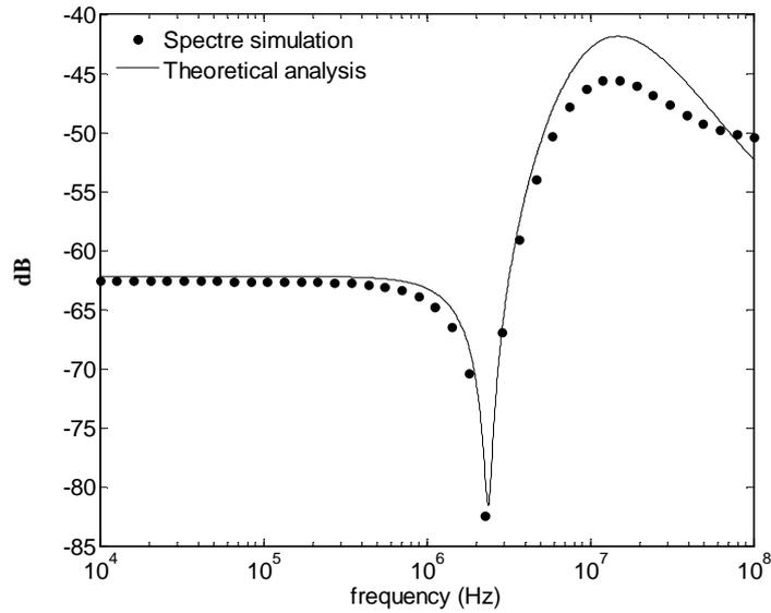
Figure 5. Third-order distortion factor of the current-sink inverter.
