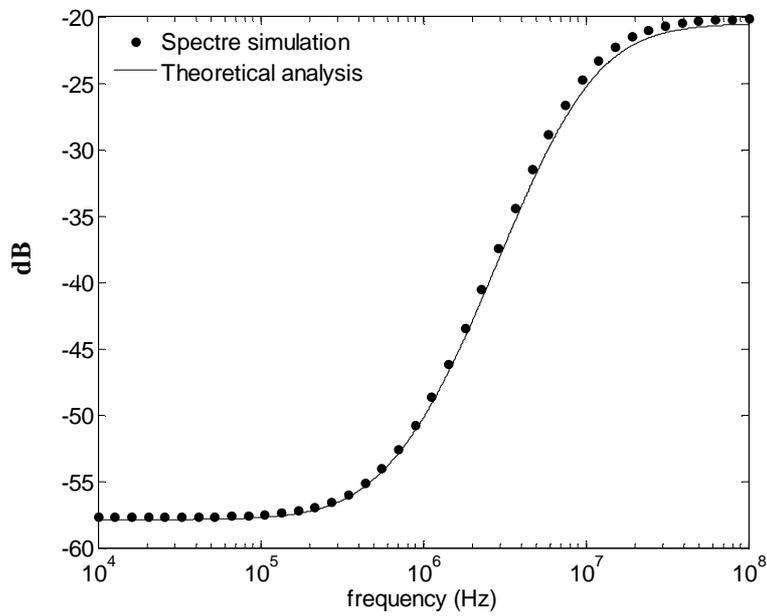
**Figure 4.** Second-order distortion factor of the current-sink inverter.
