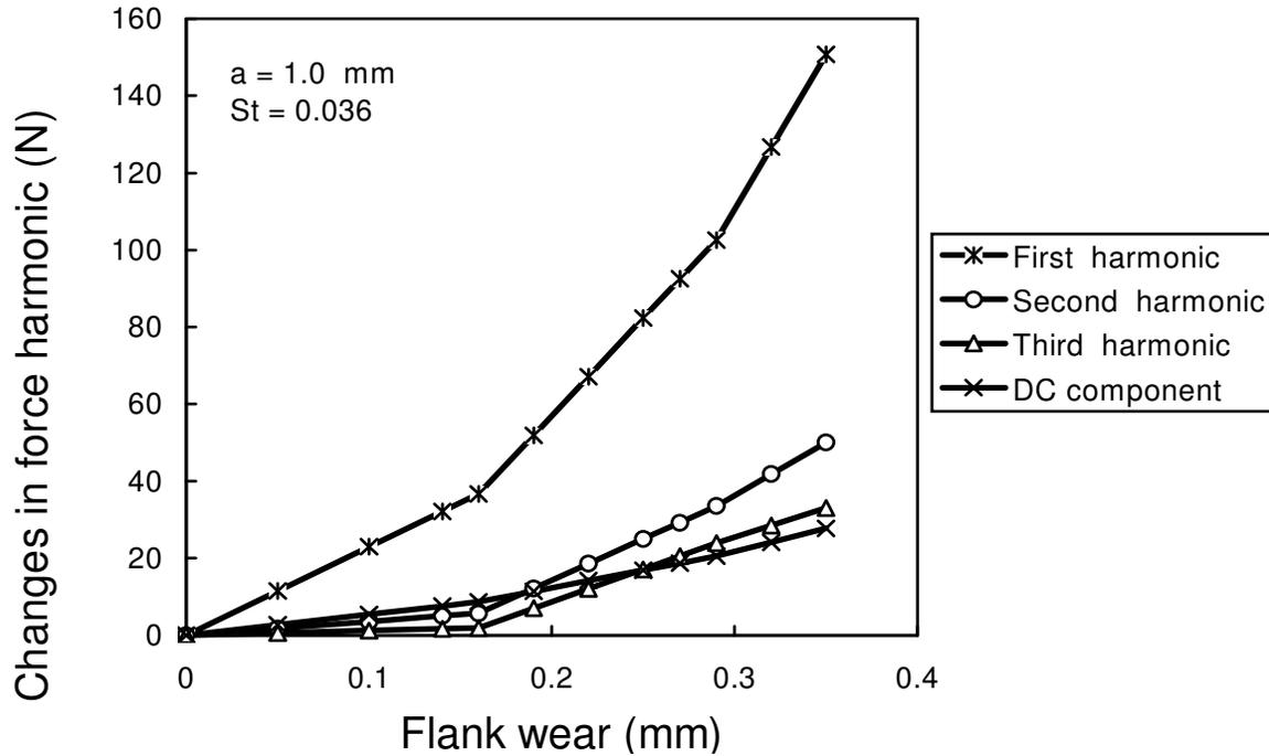
Figure 6. The change of the cutting force harmonics with tool flank wears.
