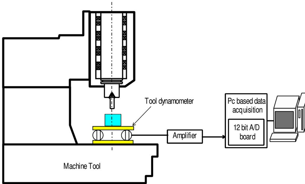
Figure 1. Schematic view of the monitoring system.
