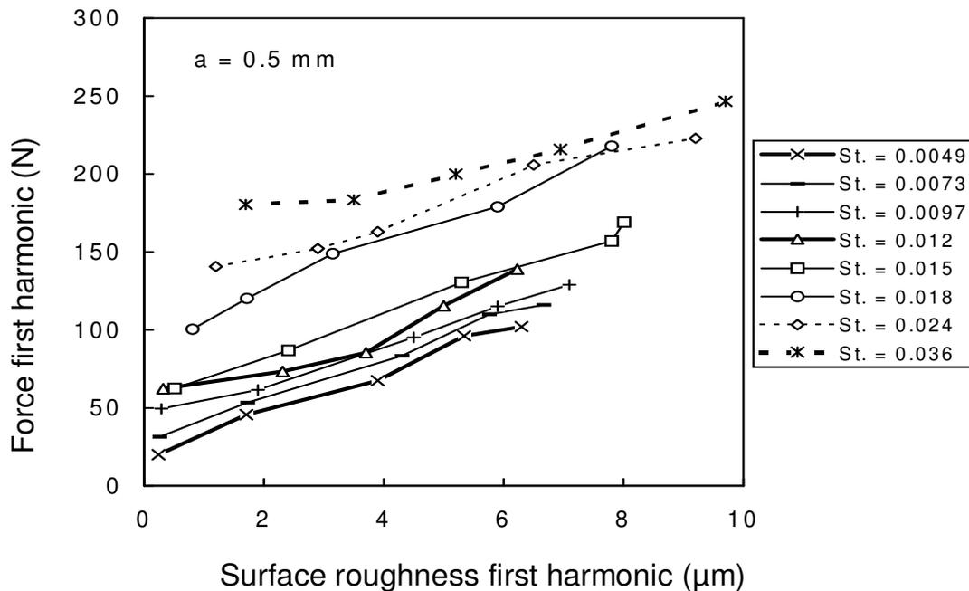
Figure 10. The relation between the cutting force first harmonic and the surface roughness first harmonic.
