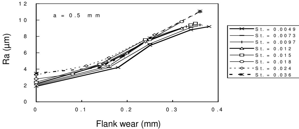
Figure 8. The effects of the tool wear change on the mean line average of the surface roughness (Ra).
