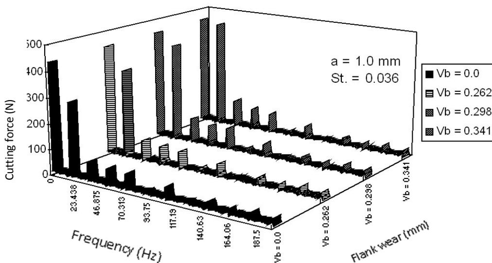
(b)  $a = 1.0$  mm**Figure 3.** An example of the estimated cutting forces in frequency domain ( $St = 0.036$  mm/tooth).
