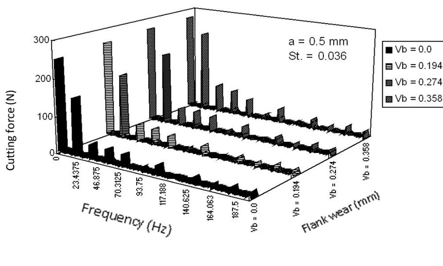
(a)  $a = 0.5$  mm
