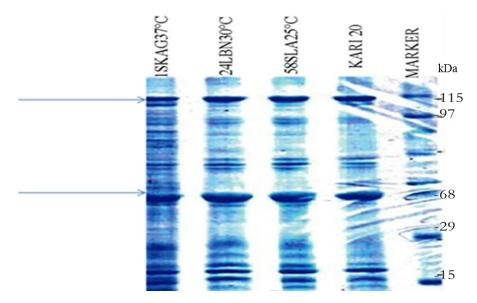
**Figure 2.** The protein bands (arrows) of delta-endotoxin and spore mixture of *Bt* isolates during its fermentation from Legume medium (1SKAG37°C and 24LBN30°C) and NYSM medium (58SLA25°C and *Bt* 20) as determined by SDS-PAGE.
