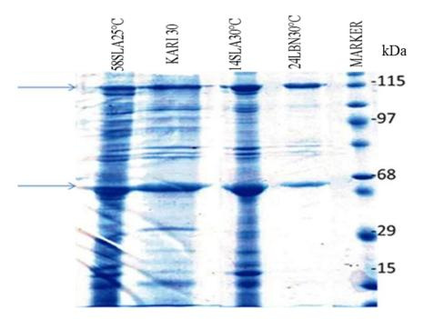
Figure 3. The protein bands (arrows) of delta-endotoxin and spore mixture of *Bt* isolates during its fermentation
