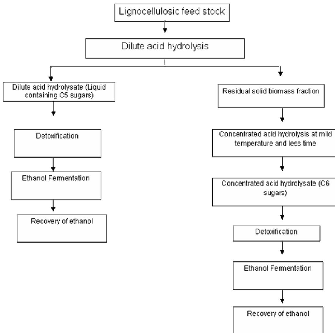
**Figure 2.** Concentrated acid hydrolysis and separate pentose and hexose sugars fermentation.
