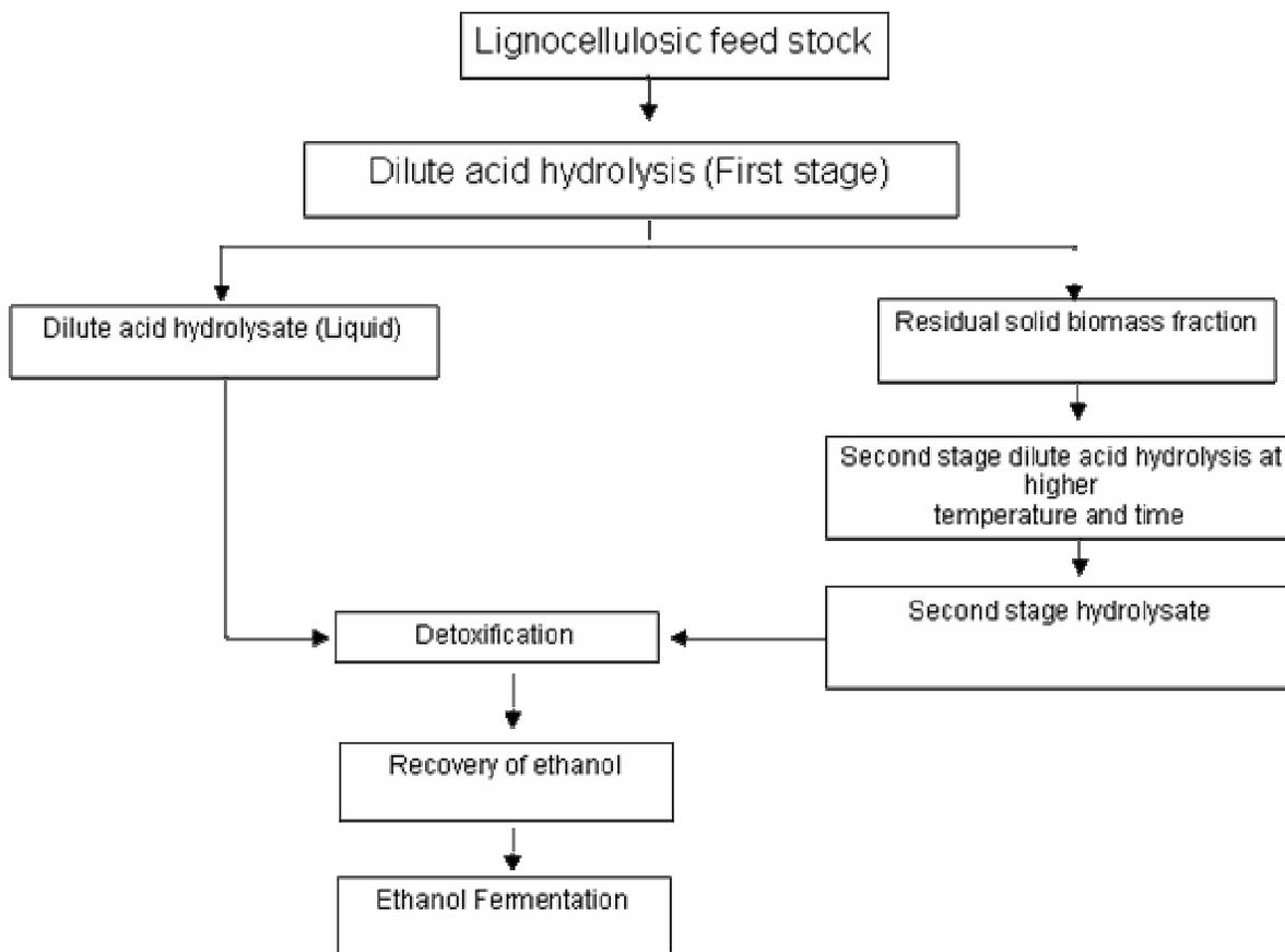
**Figure 1.** Dilute acid hydrolysis (First-stage and Two-stages) and separate fermentation of pentose and hexose sugars.
