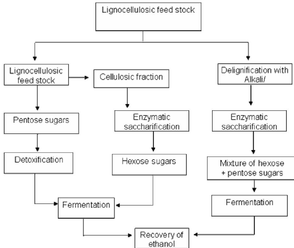
**Figure 3.** SHF with separate pentose and hexose sugars and combined sugar fermentation.
