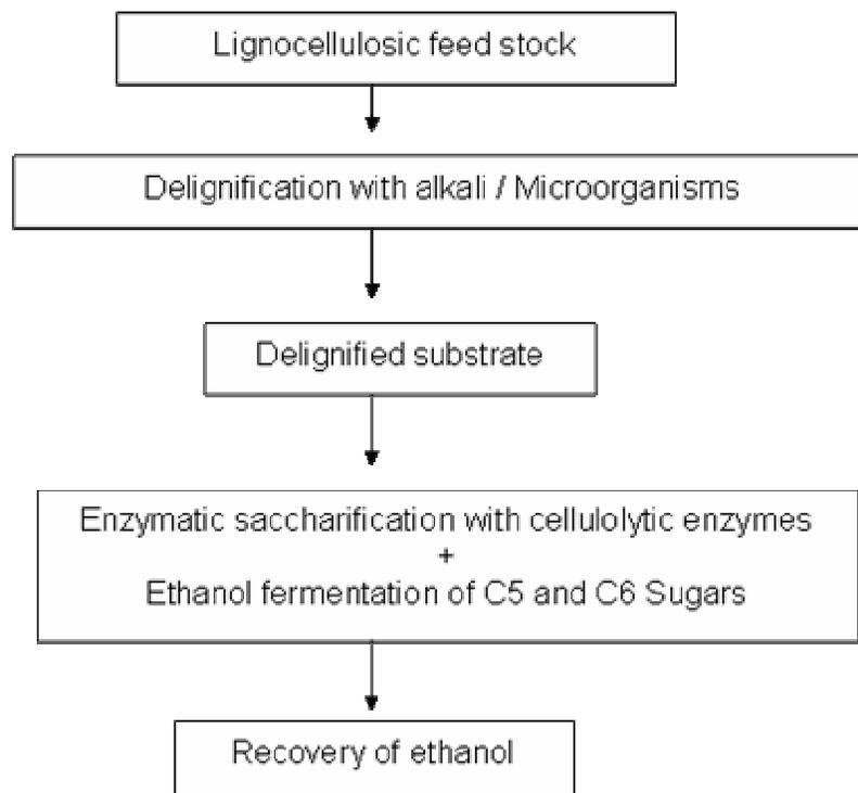
**Figure 4.** SSF with combined sugars (pentoses and hexoses) fermentation.
