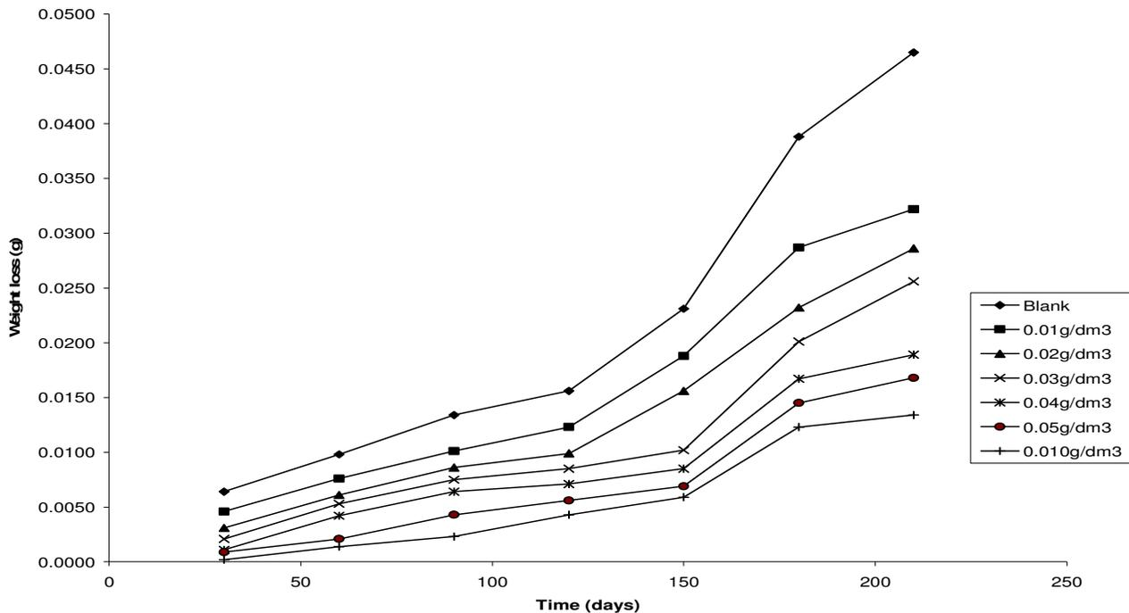
**Figure 3.** Variation of weight loss with time for zinc coupons in 2.0 M HCl solution containing different concentrations of *Aloe vera* at 30°C.
