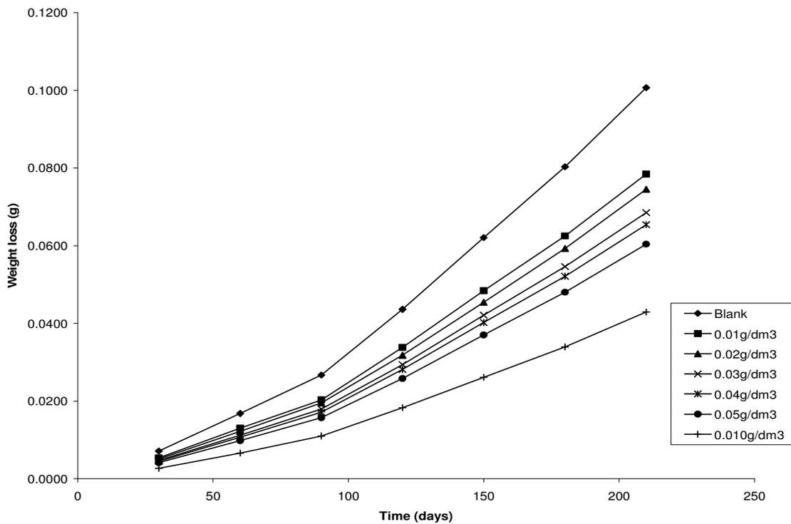
**Figure 5.** Variation of weight loss with time for zinc coupons in 2.0 M HCl solution containing different concentrations of *Aloe vera* at 50°C.
