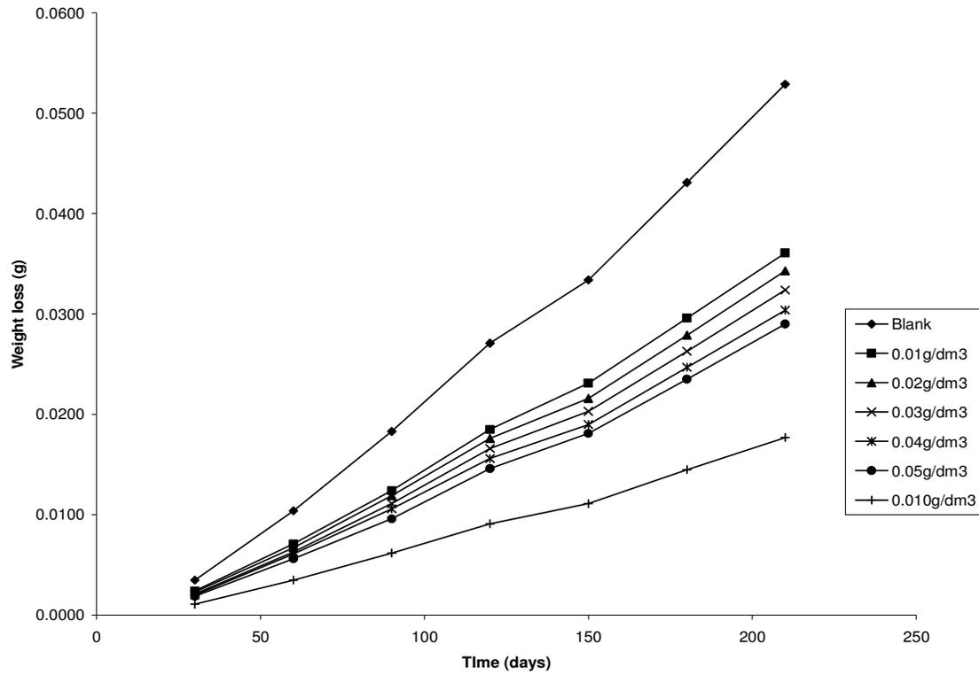
**Figure 4.** Variation of weight loss with time for zinc coupons in 2.0 M HCl solution containing different concentrations of *Aloe vera* at 40°C.
