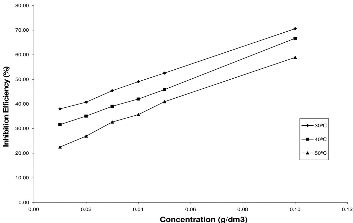
**Figure 6.** Variation of inhibition efficiency with inhibitor concentration for zinc coupons in 2.0 M HCl solution containing *Aloe vera* gel at three different temperatures.
