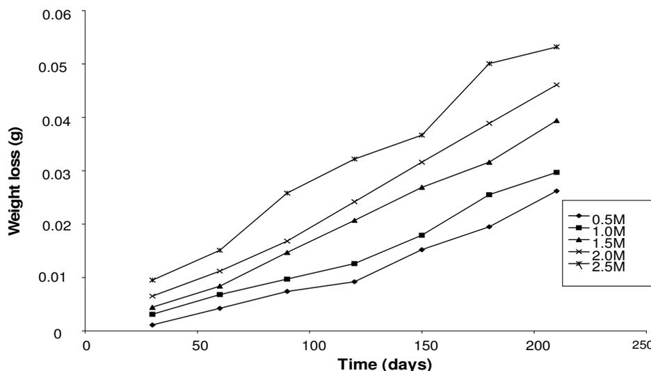
**Figure 1.** Variation of weight loss (grams) of zinc with time (days) for different concentrations of HCl solution at 30°C.
