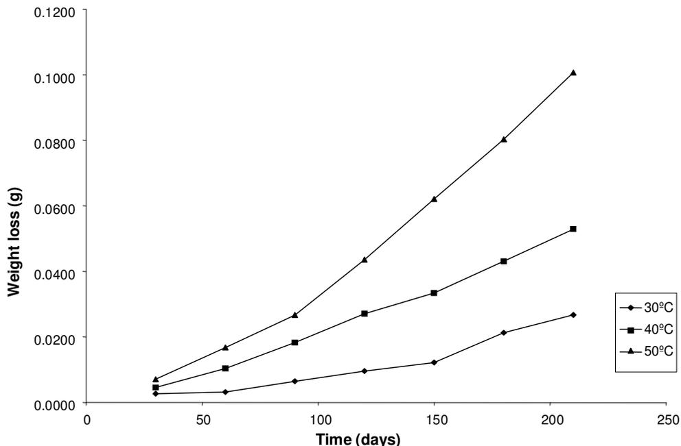
**Figure 2.** Variation of weight loss with time for zinc coupons in 2.0 M hydrochloric acid solution at three different temperatures Without *Aloe vera*.
