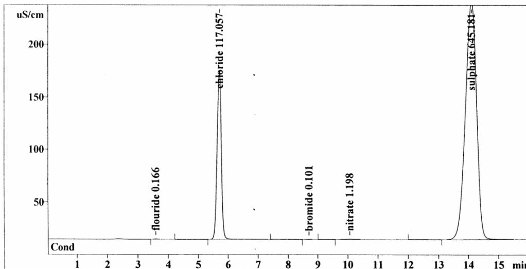
Figure 3. Chromatogram of common anions in raw water sample for Wathba plant.
