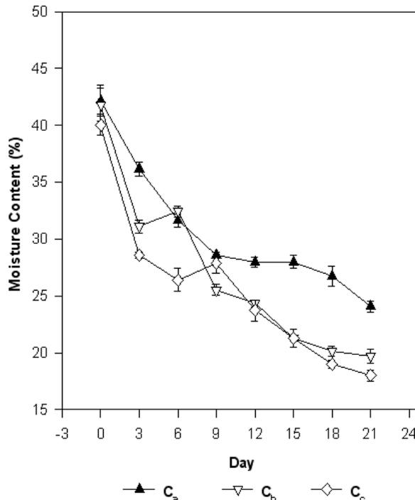
**Figure 2.** Changes of Moisture Content during Composting Processes.  $C_a$  = Oil palm frond compost A,  $C_b$  = Oil palm frond compost B,  $C_c$  = Oil palm frond compost C and  $\bar{\text{I}}$  = Standard deviation.
