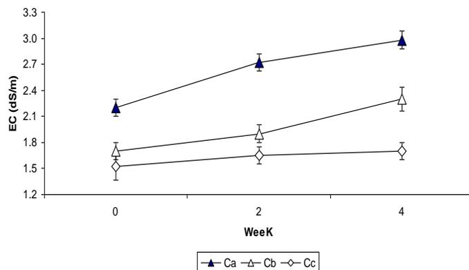
**Figure 3.** Changes of Salinity (dS/m) During Composting Processes.  $C_a$  = Oil palm frond compost A,  $C_b$  = Oil palm frond compost B,  $C_c$  = Oil palm frond compost C and  $\bar{\pm}$  = Standard deviation.
