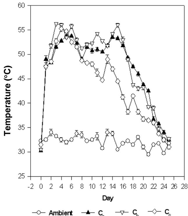
**Figure 1.** Changes in temperature ( $^{\circ}\text{C}$ ) during composting processes.  $C_a$  = Oil palm frond compost A,  $C_b$  = Oil palm frond compost B,  $C_c$  = Oil palm frond compost C and  $\bar{\text{I}}$  = Standard deviation.
