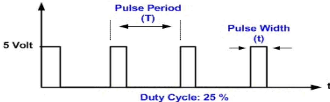
Figure 1. Pulse with 25% duty cycle.
