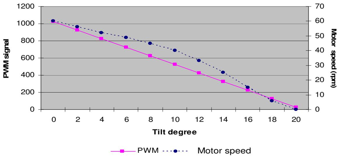
Figure 5. Chart of changes of motor speed and PWM signal to tilt degree ratio.
