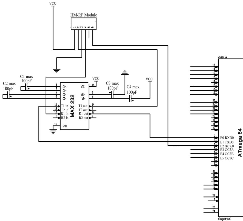
**Figure 2.** Electronic circuit for transmitting data from HM\_RF module to microcontroller.
