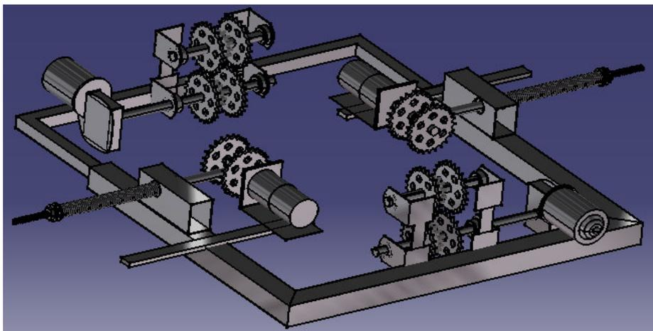
**Figure 3.** Climbing robot for oil palm tree.
