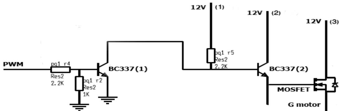
Figure 4. Electronic circuit for switching the DC motors on and off.
