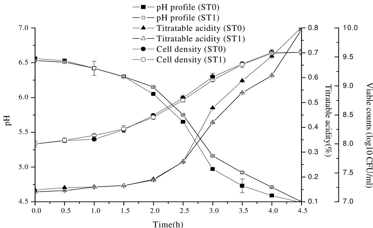
**Figure 1.** Changes in pH, titratable acidity and viable counts of fermented skim milk by ST0 and ST1 at 42°C.
