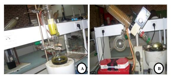
Figure 4. Soxhlet extraction assembly of (A) plant crude extracts and (B) solvents recovery.
