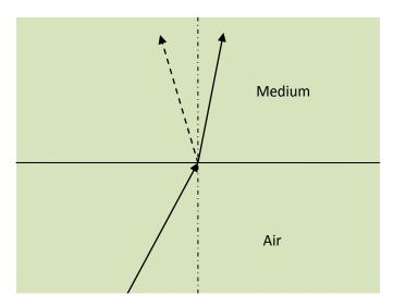
**Figure 1.** Conventional (solid) and metamaterial (dotted) refraction characteristics.
