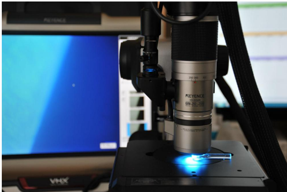
Figure 6. An example setup of digital microscopy measurement in cross-sectional view.
