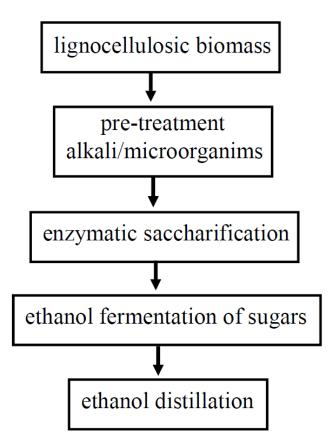
**Figure 6.** Scheme of bioethanol production by alcoholic fermentation of lignocellulosic biomass (modified from Chandel et al., 2007).
