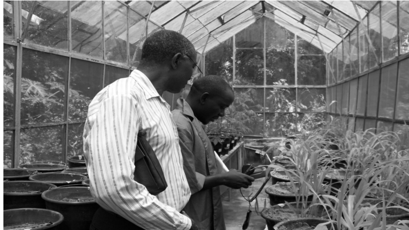
Figure 8. Recording light transmission inside the greenhouse.
