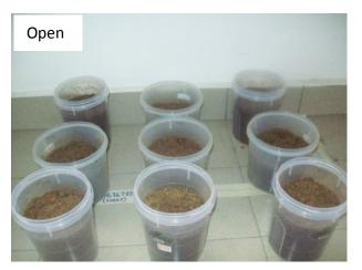
50.82% TOC and 1.46% TKN), and SD (19.32% moisture, 53.39% TOC and 0.27% TKN). The substrate to water ratio of 30:70% was used to maintain the optimum moisture content that is peculiar to SSB within the range of 50 and 60% (Haug, 1993; Sherman, 2005). Nutrients (gkg-1) of K2HPO4 (0.3), NaCl (0.3) and MgSO4.7H2O (0.3) were added to substrate as starter dose for activation of inoculated (*P. chrysosporium*) fungi. Sawdust was also added as a cheap source of carbon (Adhikari et al., 2008).
