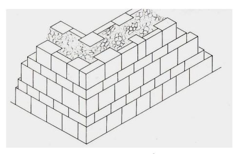
**Figure 17.** Isa Bey Mosque, Selçuk (Western Turkey), 14<sup>th</sup> century, section axonometrics indicating the rubble stone infill covered on two faces with clear-cut stone units with regular leveling courses (Aktuğ-Kolay, 1999: 26).
