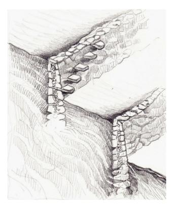
**Figure 1.** Section-axonometric drawing, retaining wall with built-in stairs in the rural settlements of the Taurus Mountains, southwestern Turkey [Construction date: mid 20th century / documented in 2009 / drawing by Kavas (2012)].
