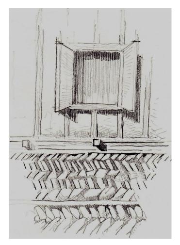
**Figure 15.** "Herring bone" technique observed in the ground floor of a traditional dwelling with a timber frame second floor, Safranbolu, northwestern Turkey (Construction date: Late Ottoman period, 19<sup>th</sup> century / drawing by Kavas (2012).
