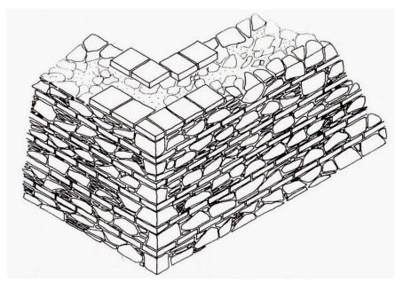
**Figure 18.** Section-axonometrics indicating the combination of stone and brick with regular leveling courses, tomb structure in Karahasan Mosque, Tire, Western Turkey (Construction date: 14<sup>th</sup> century / reference: Aktuğ-Kolay, 1999: 29).
