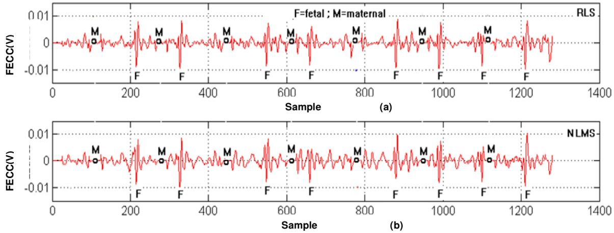
**Figure 10.** Fetal signal after the IIR notch filter, (a) fetal extracted signal by RLS filter, (b) fetal extracted signal by NLMS filter (M = locations of maternal signal peaks and F = fetal signal peaks).
