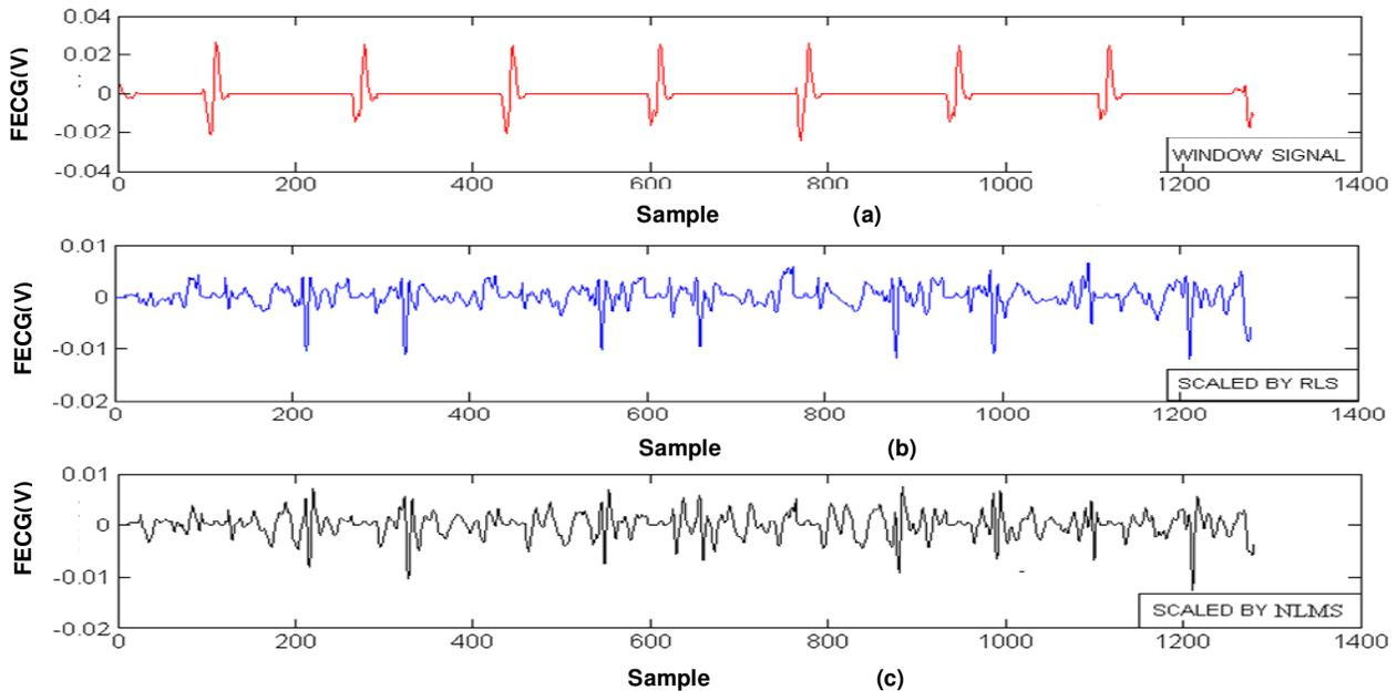
**Figure 9.** (a) The window signal, (b) scaled fetal extracted signal by RLS filter and (c) scaled fetal extracted signal by NLMS filter.
