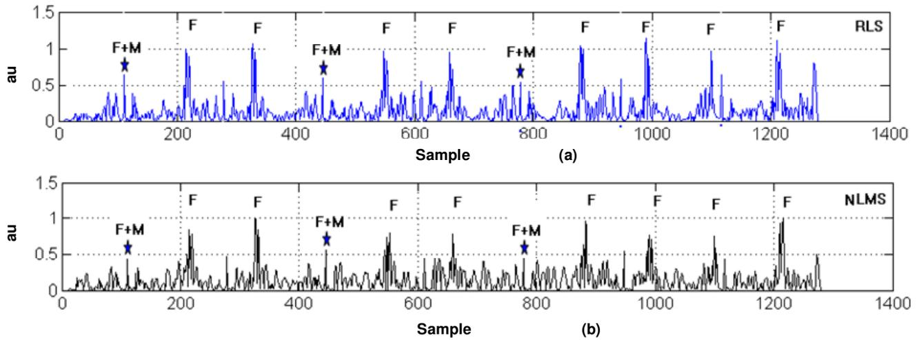
**Figure 11.** Fetal signal after adjustment, (a) fetal extracted signal by RLS filter, (b) fetal extracted signal by NLMS filter (F = fetal signal peaks and F + M = overlapped peaks).
