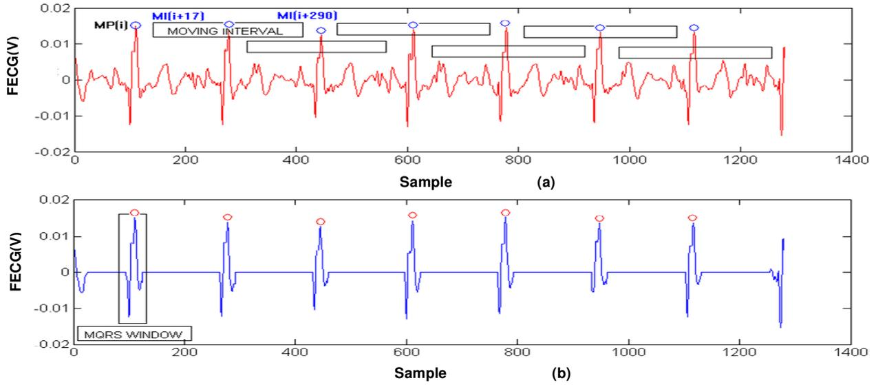
Figure 4. (a) Peak detection using MI, (b) window signal consisting of seven MQRS windows.
