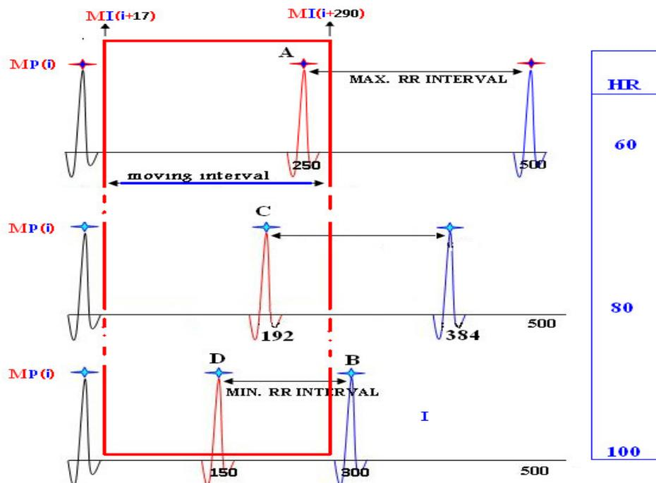
Figure 3. Moving interval for peak detection.
