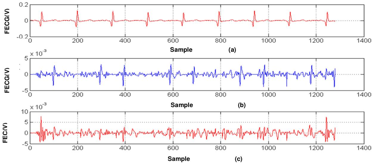
**Figure 8.** (a) Primary signal after preprocessing stage showing negligible fetal signal, (b) fetal extracted signal by RLS filter, and (c) fetal extracted signal by NLMS filter.
