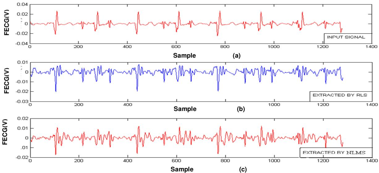
**Figure 7.** (a) Primary signal after preprocessing stage, (b) fetal extracted signal by RLS filter and (c) fetal extracted signal by NLMS filter.
