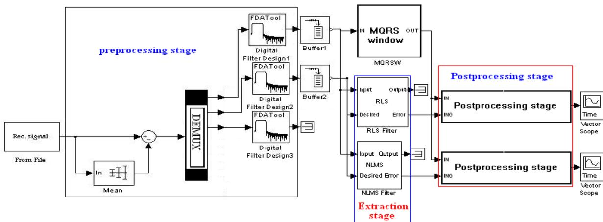
Figure 6. Computer simulation for FECG extraction using RLS and NLMS filters.
