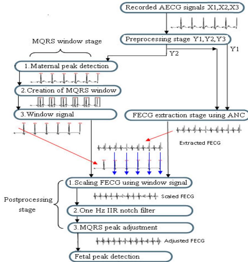
Figure 2. The block diagram of the proposed technique.
