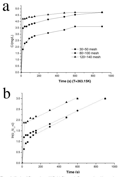
**Figure 3.** Kinetics of F extraction at 90°C. (a) Changes in F concentration with extraction time; (b) Functional relationship of  $\ln[c_{\infty}/(c_{\infty}-c)]$  with time. Particle mean size:  $\blacktriangle$ , 0.113 mm; •, 0.160 mm; •, 0.380 mm.
