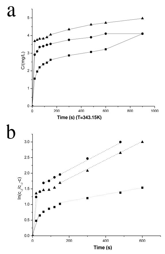
**Figure 2.** Kinetics of F extraction at 70°C. a: Changes in F concentration with extraction time; b: Functional relationship of  $\ln[c_{\infty}/(c_{\infty}-c)]$  with time. Particle mean size:  $\blacktriangle$ , 0.113 mm;  $\bullet$ , 0.160 mm;  $\blacksquare$ , 0.380 mm.
