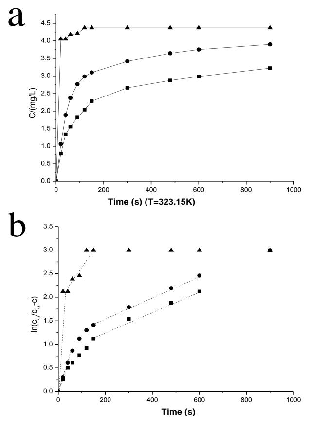
**Figure 1.** Kinetics of F extraction at 50°C. a: Changes in F concentration with extraction time; b: Functional relationship of  $\ln[c_{\omega}/(c_{\omega}-c)]$  with time. Particle mean size:  $\blacktriangle$ , 0.113 mm;  $\bullet$ , 0.160 mm;  $\blacksquare$ , 0.380 mm.
