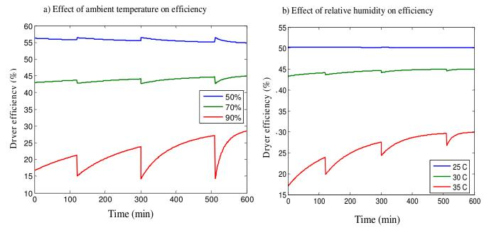
Figure 8. Effect of operating conditions on the drying effeciency.
