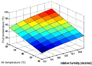
a) Effect of air temperature and humidity on fruit temperature
