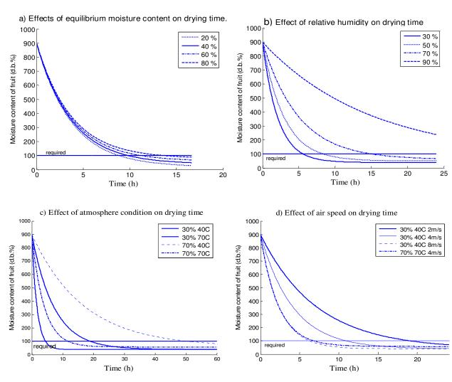
Figure 4. Effect of different parameters on the drying time.
