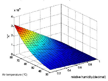
**Figure 5.** Effects of air temperature and humidity on fruit temperature and 'k'.
