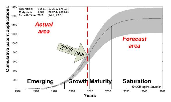
Figure 5. The growth curve of SOFC technology by using the logistic model: the number of publications.
