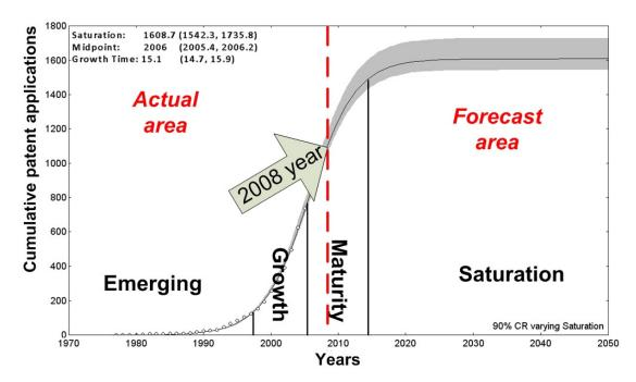
Figure 4. The growth curve of PEMFC technology by using the logistic model: the number of publications.
