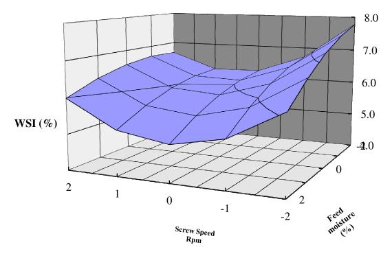
Figure 2. Effect of screw speed and feed moisture on WSI.
