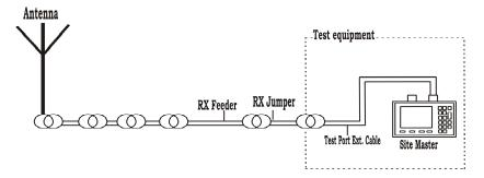
Figure 1. Measurement setup of Anritsu site master instrument.
