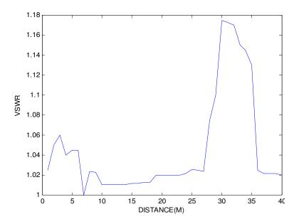
**Figure 2.** A graph of VSWR versus distance in Evbotubu district base station in Benin City.
