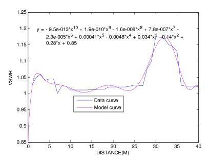
Figure 3. A Model graph of VSWR versus distance.
