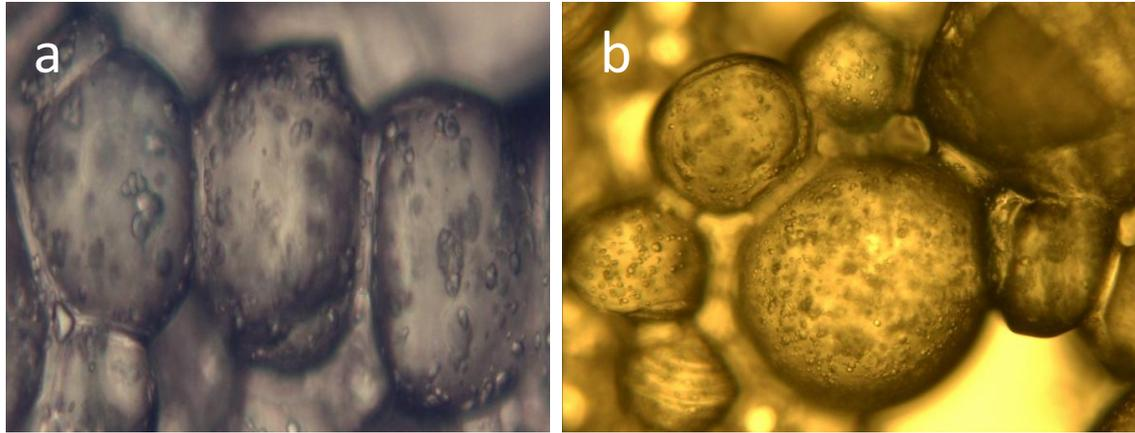
**Figure 1.** Optical microscope image of coated alginate-resistant starch capsule (a and b) at 40x magnification.
