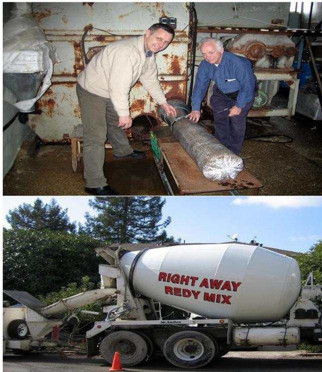
**Figure 3.** Top: Mr. Gusev demonstrates the way his mixing machine fills polyethylene tubes with the pasteurized, spawned substrate. Bottom: A concrete mixer that might be used for a pasteurization mixer. These are often available for used.
