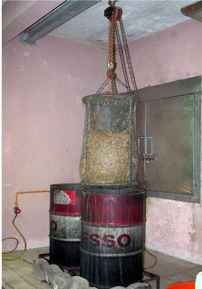
**Figure 2.** Steel drums on gasburners with wire basket and chain-fall. This arrangement and one ton of dry waste-substrate (the tons of wet) in a day.
