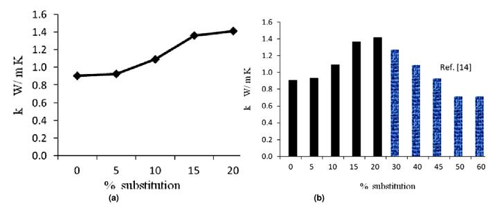
Figure 7. Plot of thermal conductivity against percentage RHA substitution for (a) 0-20; (b) 0-60.
