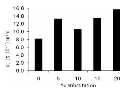
Figure 9. Plot of thermal diffusivity against percentage RHA substitution.
