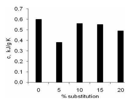
Figure 8. Plot of specific heat capacity against percentage RHA substitution.
