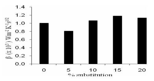
Figure 10. Plot of thermal effusivity against percentage RHA substitution.
