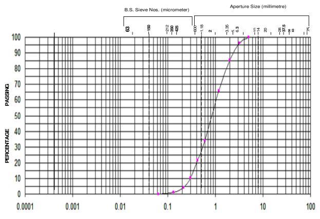
Figure 1. Particle size distribution curve of sand.
