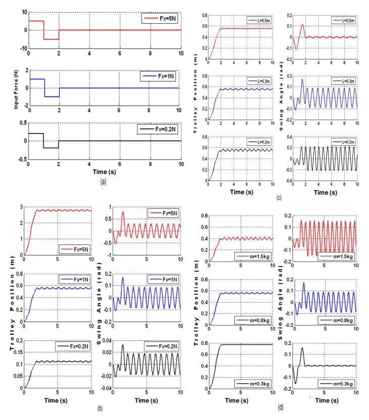
**Figure 3.** (a) Bang-bang with different input forces 1, 5 and 0.2 N. (b) Trolley position and swinging angle at different Fx. (c) Trolley position and swinging angle with different rope length (L= 0.2, 0.3 and 0.5 m). (d) Trolley position and swinging angle with different load masses (m= 0.3, 0.8 and 1.5 kg).
