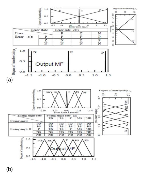
Figure 6. (a) Fuzzy sets for the proposed fuzzy PD-based position control (b) and either anti-swing compensator.
