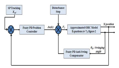
Figure 4. Proposed fuzzy PD-based overhead control system.
