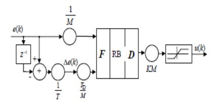
Figure 5. Fuzzy PD controller structure with the normalized universe range.
