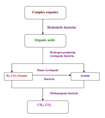
Figure 2. Biogas production process (Omer, 2003).
