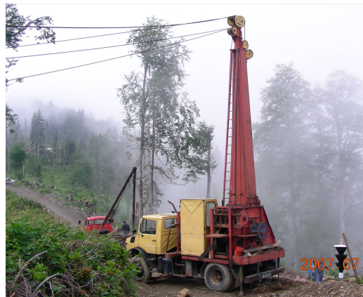
Figure 1. Urus Mill cable crane in felling area.
