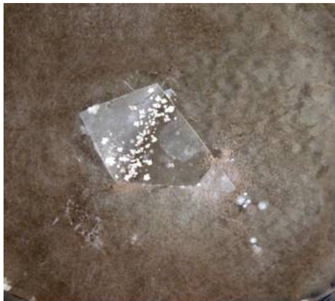
Figure 1. The visible growth of microbial consortia growing on expanded polystyrene film used for isolation of bacteria.
