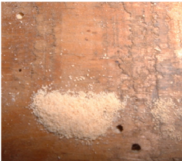
Figure 1. Small pile of dust accumulates near exit holes of A. punctatum in the wood.
