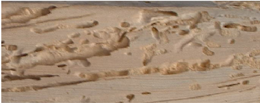
Figure 3. Damages of H. bajulus (L.).
